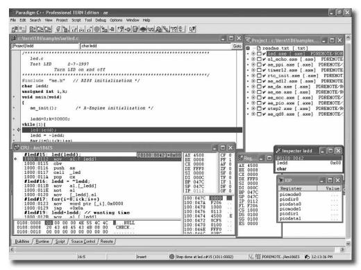
You can see the development system in action on the page 5 screen-shot. This screen-shot shows the sample program *led.c* being debugged. This basic C program, which blinks the LED, is running directly on the TERN controller while the debugger retains full control over the execution.
