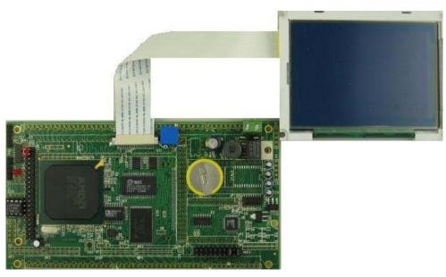
Figure 3.7 586D controller with LCD cable interface.
