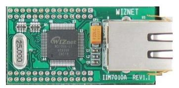
Figure 3.8 WizNet™ Ethernet Module
