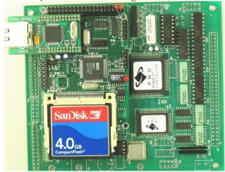
A CAN-Engine<sup>TM</sup> installed on the top of a MotionC board.
