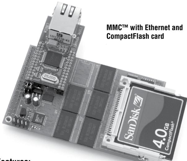
**MMC™ with Ethernet and CompactFlash card**
