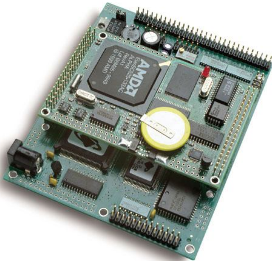
Figure 1.3 A 586-Engine installed on the MotionC2140
