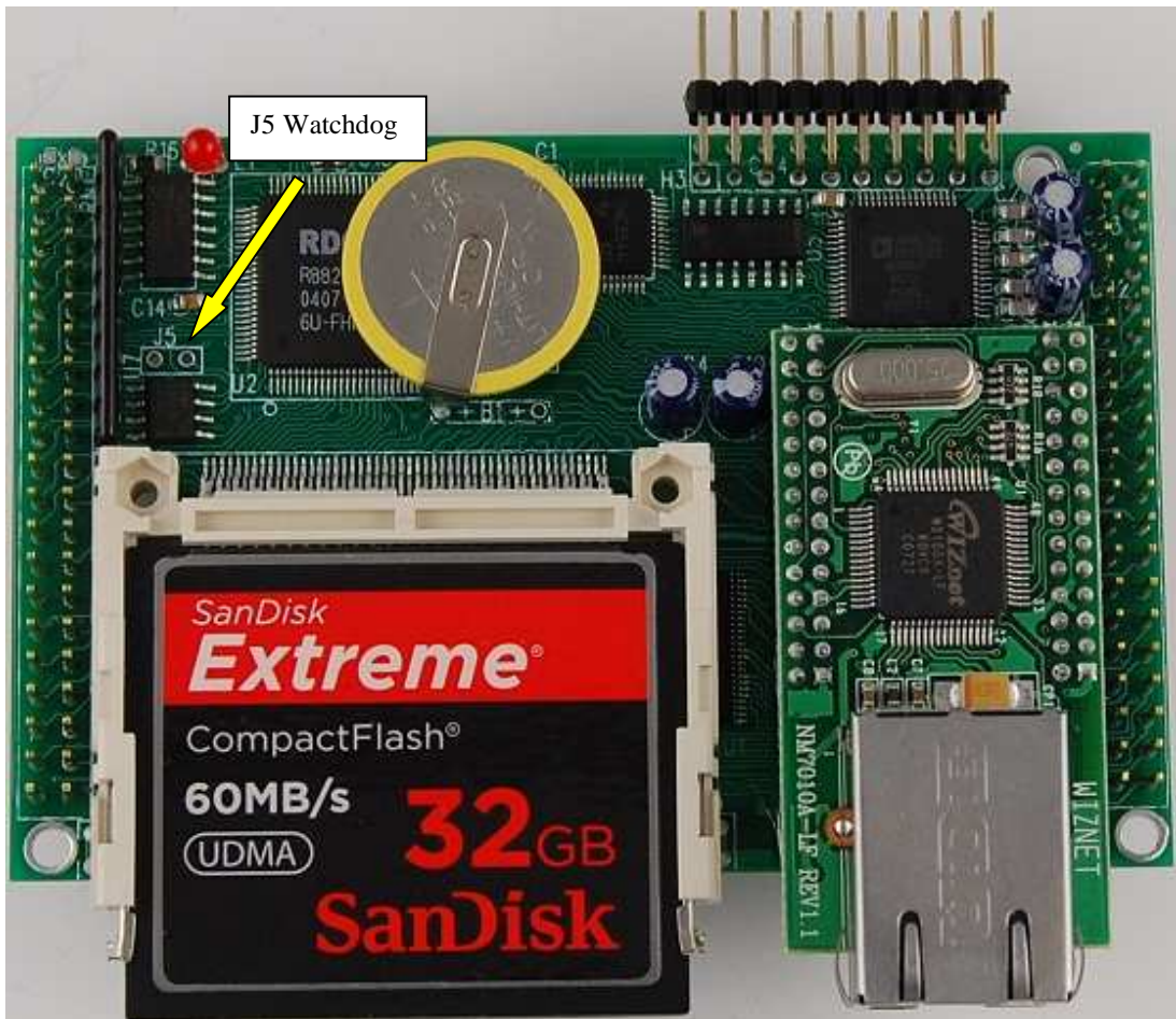
Figure 3.1 Location of watchdog timer enable jumper
