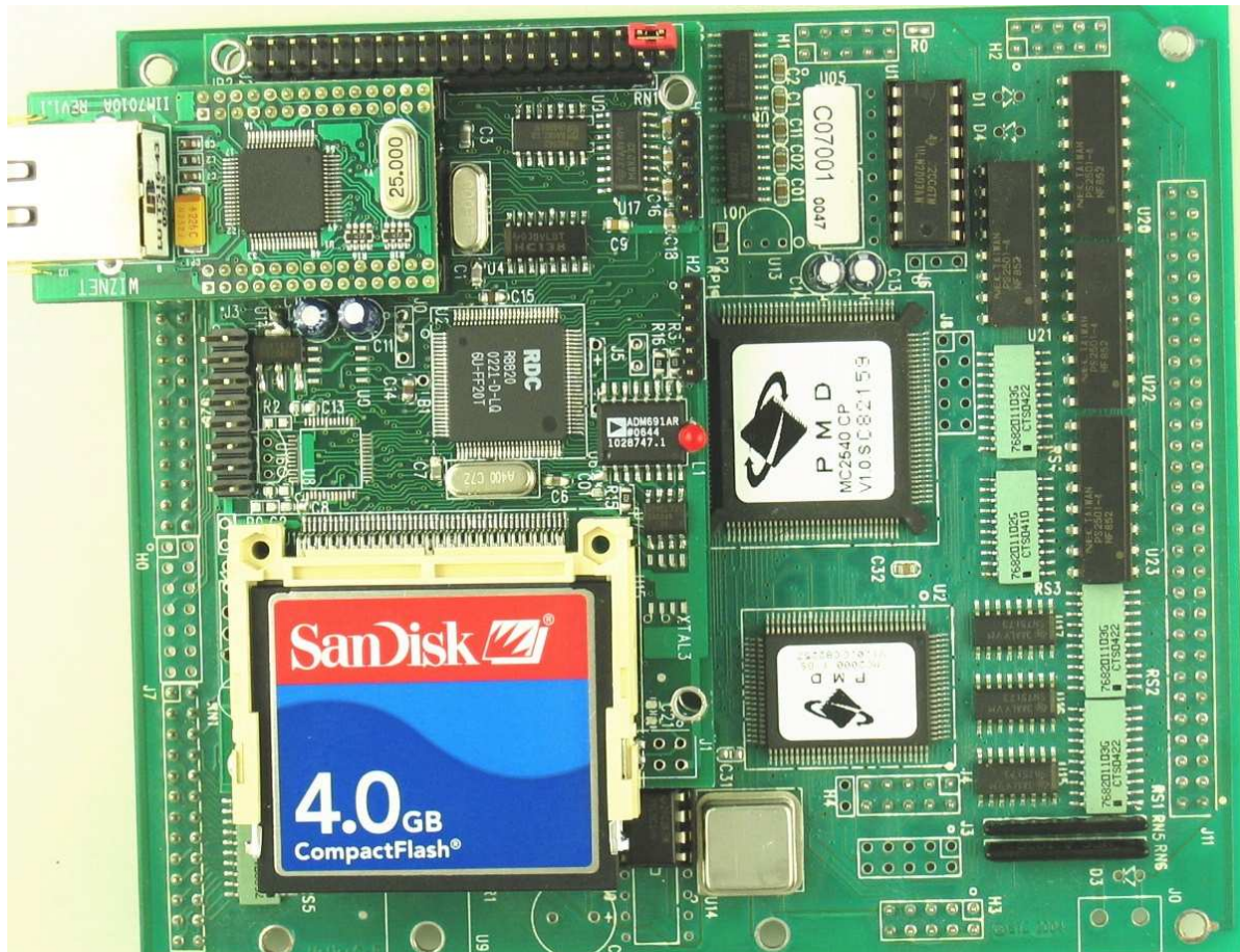
Figure 1.4 CAN-Engine is installed on the top of the MotionC-P.
