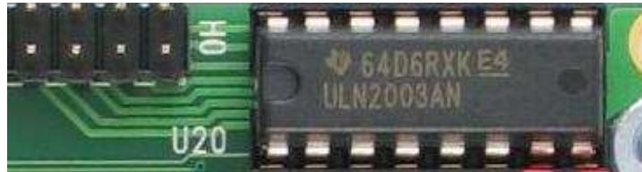
Figure 3.3 High Voltage Driver w/ H0 header output pins
