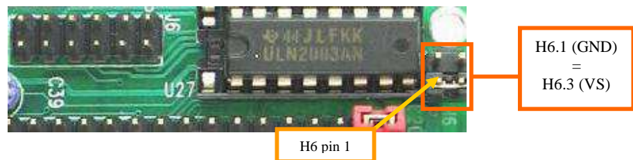
Figure 3.2 High Voltage Driver w/ J6 header sinking output pins
