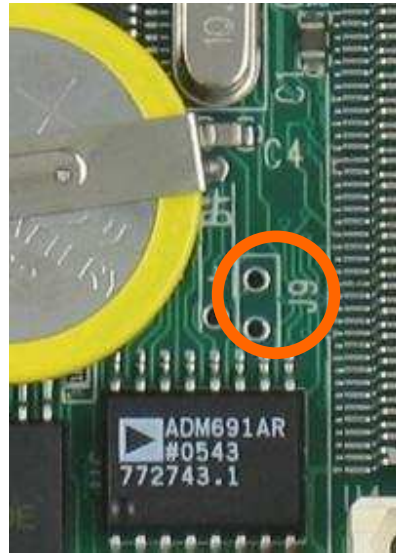
Figure 3.3 Location of watchdog timer enable jumper
