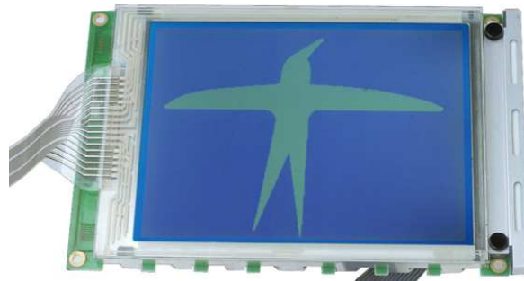
Figure 1.2 Front view of the SmartLCD: 320x240 graphic LCD displaying bird
