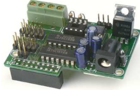
Figure 1.2 VE232 interface board
